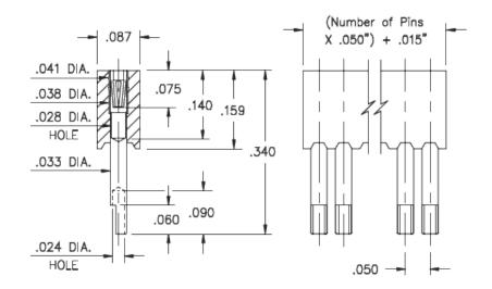
**Description:** Interconnect Socket Solder Cup Strip Socket Accepts .015"- .020" (0,38 - 0,508 mm) dia leads Single Row Through Hole
