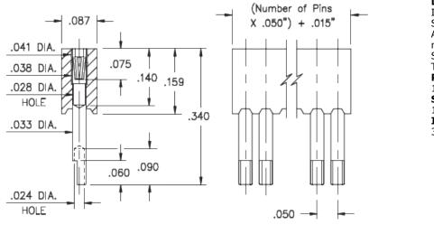
Description: Interconnect Socket Solder Cup Strip Socket Accepts .015"- .020" (0,38 - 0,508 mm) dia leads Single Row Through Hole **Plating Code:** 13
