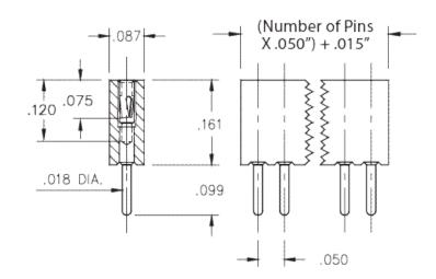
Interconnect Socket Standard Solder Tail Socket Accepts .015"- .020" (0,38 - 0,508 mm) dia leads Single Row Through Hole Plating Code: 41 Shell Plating: 200 µ" Tin (matte finish) over 100 µ" Nickel Inner Contact Plating: 10 µ" Gold over 50 µ" Nickel
