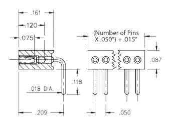
**Description:** Interconnect Socket Right Angle Socket Accepts .015"- .020" (0,38 - 0,508 mm) dia leads Single Row Through Hole Plating Code: **Shell Plating:** 200 μ" Tin/Lead(93/7) over 100 μ"
