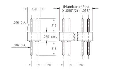
**Description:** Interconnect Header Solder Tail Pin Header .016" (0,41mm) Pin Head Double Row Through Hole Plating Code: 10 Shell Plating: 10  $\mu$ " Gold over 100  $\mu$ " Nickel
