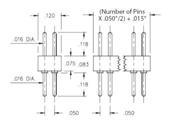
**Description:** Interconnect Header Solder Tail Pin Header .016" (0,41mm) Pin Head Double Row Through Hole Plating Code: 90 Shell Plating:
