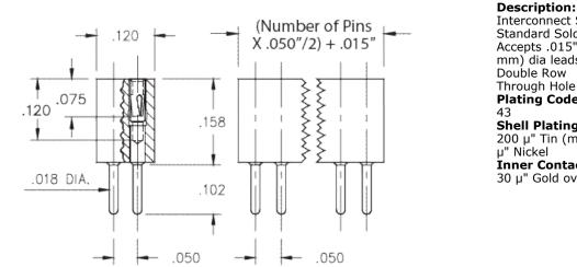
Interconnect Socket Standard Solder Tail Socket Accepts .015"- .020" (0,38 - 0,508 mm) dia leads Double Row Through Hole Plating Code: 43 Shell Plating: 200 µ" Tin (matte finish) over 100 µ" Nickel Inner Contact Plating: 30 µ" Gold over 50 µ" Nickel
