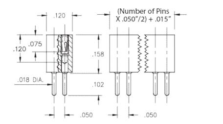
Interconnect Socket Standard Solder Tail Socket Accepts .015"- .020" (0,38 - 0,508 mm) dia leads Double Row Through Hole Plating Code: 43 Shell Plating: 200 µ" Tin (matte finish) over 100 µ" Nickel Inner Contact Plating: 30 µ" Gold over 50 µ" Nickel
