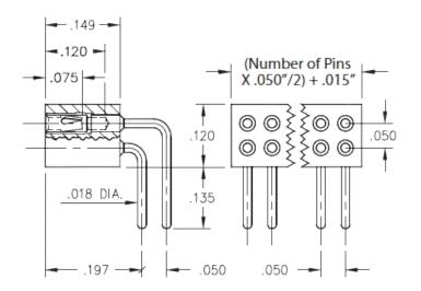
**Description:** Interconnect Socket Right Angle Socket Accepts .015"- .020" (0,38 - 0,508 mm) dia leads
