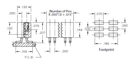
Interconnect Socket Surface Mount Socket Accepts .015"- .020" (0,38 - 0,508 mm) dia leads Double Row Plating Code: 43 Shell Plating: 200 µ" Tin (matte finish) over 100 µ" Nickel Inner Contact Plating: 30 µ" Gold over 50 µ" Nickel
