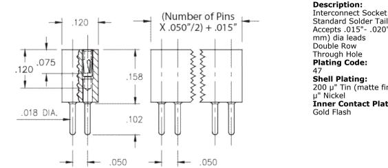
Standard Solder Tail Socket Accepts .015"- .020" (0,38 - 0,508 mm) dia leads Double Row Through Hole **Plating Code:** Shell Plating: 200 µ" Tin (matte finish) over 100 µ" Nickel Inner Contact Plating:
