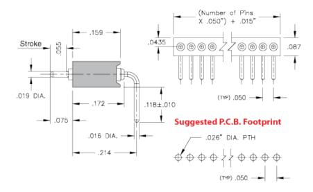
**Description:** Interconnect SLC Header Spring-Loaded Header Horizontal Mount Single Row Through Hole Plating Code: Shell Plating:
