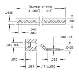
**Description:** Interconnect Target Connector Spring-Loaded Header Horizontal Mount Target Single Row Through Hole Plating Code: 10 Shell Plating: 10  $\mu$ " Gold over 100  $\mu$ " Nickel
