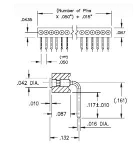
Description: Interconnect Target Connector Spring-Loaded Header Right Angle Mount Target Single Row Through Hole Plating Code: 10 Shell Plating: 10  $\mu$ " Gold over 100  $\mu$ " Nickel
