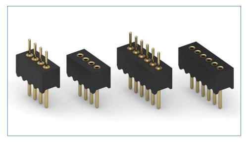
Mill-Max is pleased to announce new additions to our line of fine pitch connectors with the introduction of 1 mm pitch headers and sockets. These through-hole, single row sockets and headers are ideal for real estate saving interconnect solutions. The 860-10-0XX-10-002000 header and 861-13-0XX-10-002000 socket (XX=2 to 50) join our 1.27 mm (.050"); 1.778 mm (.070") and 2 mm (.0787") pitch interconnect offerings.
