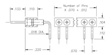
**Description:** Interconnect Header Right Angle Pin Header .019" (0,48mm) Pin Head Single Row Through Hole Plating Code: 10 Shell Plating: 10  $\mu$ " Gold over 100  $\mu$ " Nickel
