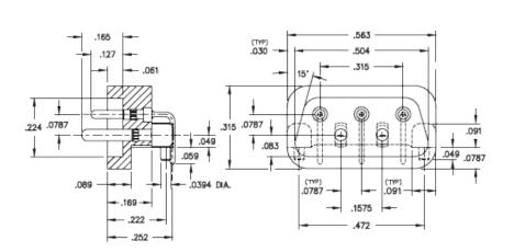
Description: Power and Signal Header Right Angle Mount Double Row Through Hole Plating Code: 30
