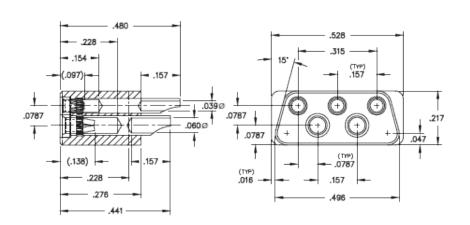
**Description:** Power and Signal Socket Solder Cup Strip Socket Double Row **Plating Code:** 93 Shell Plating: 200 μ" Tin/Lead(93/7) over 100 μ" Nickel Inner Contact Plating: 30 µ" Gold over 50 µ" Nickel Packaging: Packaged in Bulk
