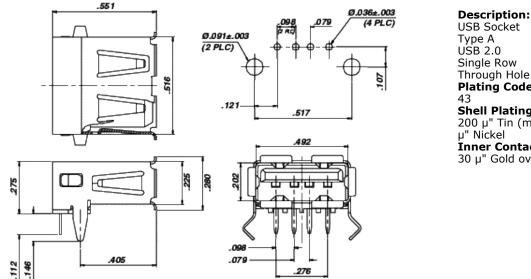
USB Socket Type A USB 2.0 Single Row Through Hole **Plating Code:** 43 **Shell Plating:** 200 µ" Tin (matte finish) over 100 µ" Nickel **Inner Contact Plating:** 30 µ" Gold over 50 µ" Nickel
