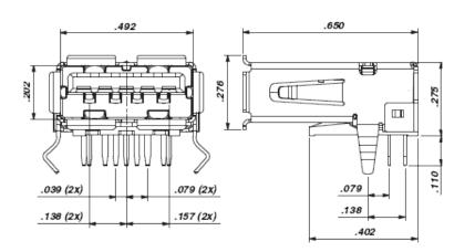
Description: USB Socket Type A USB 3.0 Single Row Through Hole Plating Code: 46 Shell Plating: Terminals: Tin Plated Inner Contact Plating: 30 μ" Gold
