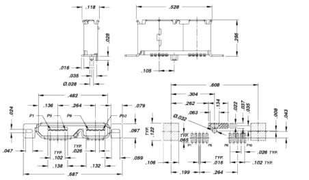
USB Socket Micro-B USB 3.0 Single Row Surface Mount **Plating Code:** 10 **Shell Plating:** 10 µ" Gold over 100 µ" Nickel **Packaging:** Tape
