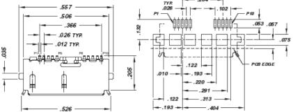
**Description:** USB Socket Micro-B USB 3.0 Surface Mount **Plating Code:** 10
