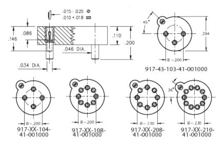
**Description:** Transistor TO Socket SMT Accepts .015" - .025" (0,38 - 0,635 mm) dia leads Surface Mount Plating Code: 43 Shell Plating: 200 μ" Tin (matte finish) over 100
