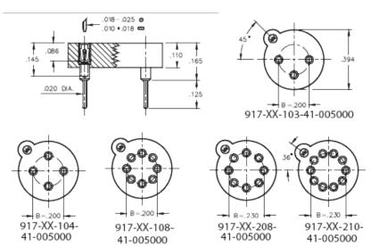
**Description:** Transistor TO Socket Through-Hole Mount Accepts .015"- .025" (0,38 - 0,635 mm) dia leads Through Hole **Plating Code:** 43
