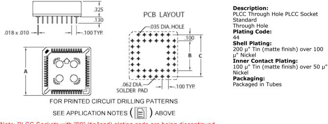
Note: PLCC Sockets with "99" (tin/lead) plating code are being discontinued and will only be available in RoHS compliant "44" (pure tin). "99" plating is still available in limited quantities until all existing stock is depleted.
