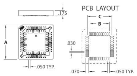
FOR PRINTED CIRCUIT DRILLING PATTERNS
