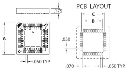
FOR PRINTED CIRCUIT DRILLING PATTERNS
