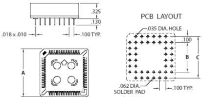
FOR PRINTED CIRCUIT DRILLING PATTERNS
