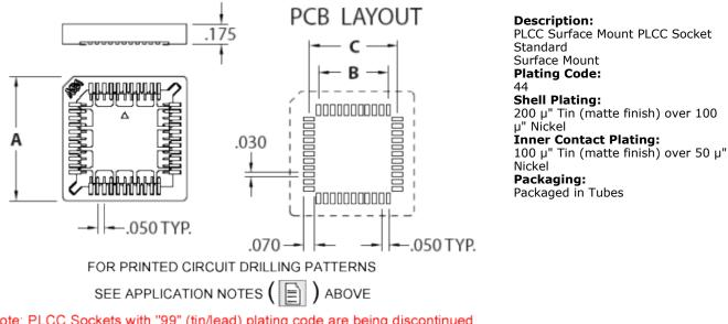
Note: PLCC Sockets with "99" (tin/lead) plating code are being discontinued and will only be available in RoHS compliant "44" (pure tin). "99" plating is still available in limited quantities until all existing stock is depleted.
