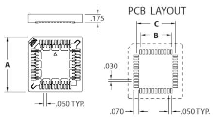
FOR PRINTED CIRCUIT DRILLING PATTERNS
