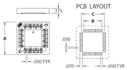
FOR PRINTED CIRCUIT DRILLING PATTERNS
