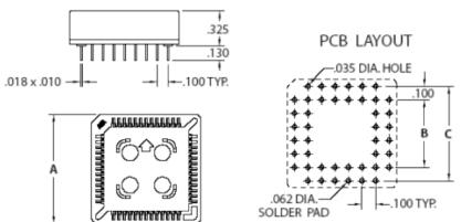
FOR PRINTED CIRCUIT DRILLING PATTERNS
