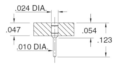
**Description:** 9929 - Press-Fit PCB Pin Packaging: Packaged in Bulk
