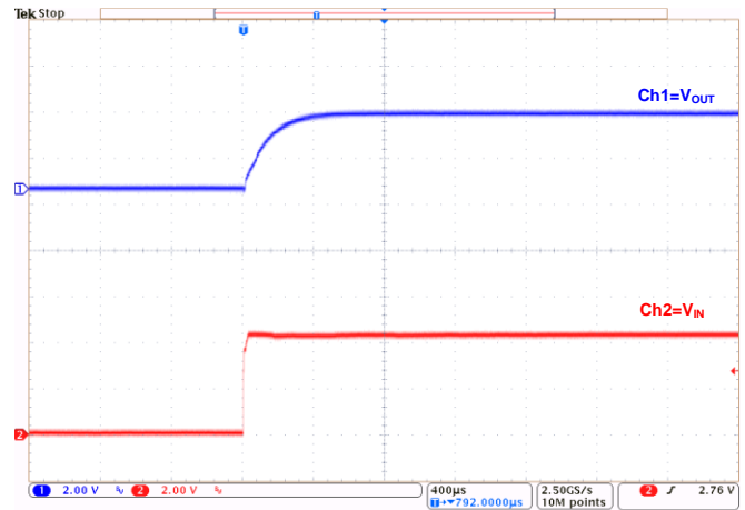
Power Up at V_{OUT}=3.3V : ( I_{OUT}=500mA )
