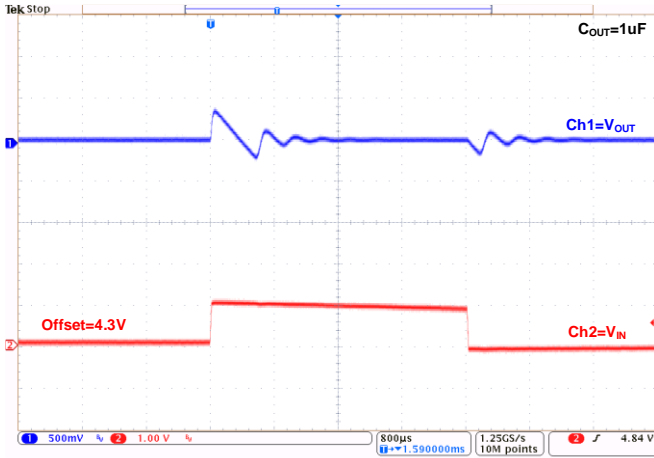
Line Transient at V_{OUT}=3.3V : ( I_{OUT}=1mA )
