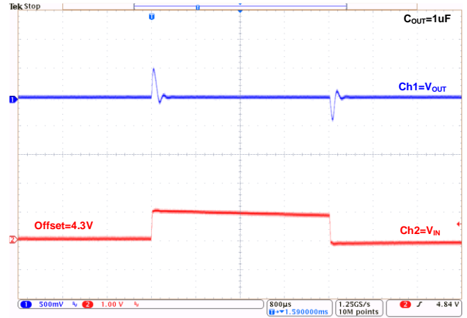
Line Transient at V_{OUT}=3.3V : ( I_{OUT}=10mA )
