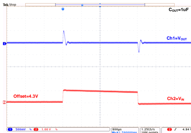
Line Transient at V_{OUT}=3.3V : ( I_{OUT}=10mA )
