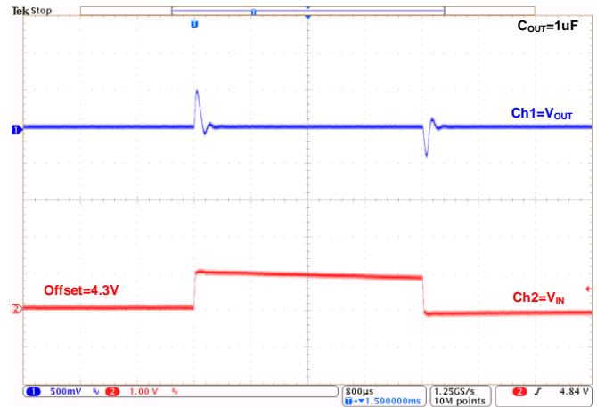
Line Transient at V_{OUT}=3.3V : ( I_{OUT}=10mA )
