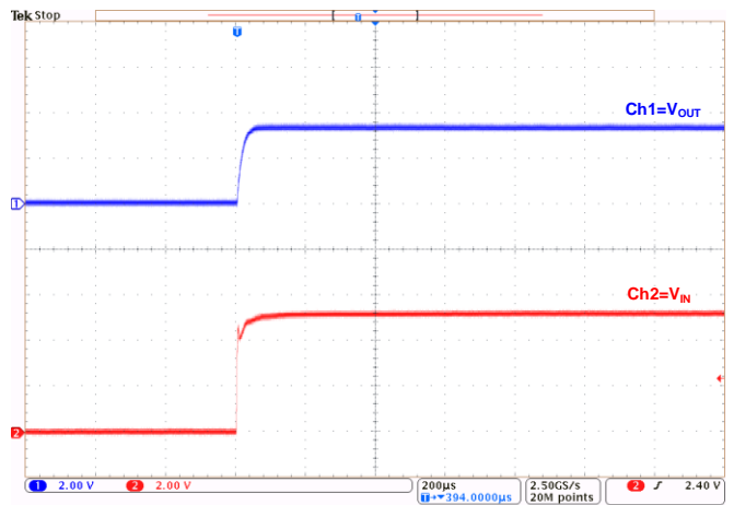
Power-Up at V_{OUT}=3.3V : ( I_{OUT}=1A )
