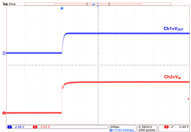
Power-Up at V_{OUT}=3.3V : ( I_{OUT}=1A )
