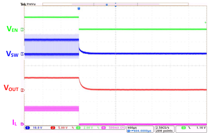
Figure 16. Shutdown Through EN, I_{OUT} = 0.6A
