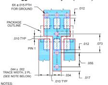
. TRACE WIDTH IS SHOWN FOR ROGERS RO4350B WITH DIELECTRIC THICKNESS .020° ± .0015°. COPPER: 1/2 OZ. EACH SIDE. FOR OTHER MATERIALS TRACE WIDTH MAY NEED TO BE MODIFIED.
