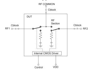
Cblock should be free of resonance over frequency of operation.
