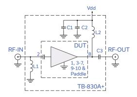
Fig 1. Application and Characterization Circuit
