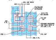
AR WAYEGUIDE PARAMETERS ARE SHOWN FOR ROGERS RO4350B ELECTRIC THICKNESS 0.020±0.0015; COPPER: 1/2 02. EACH SIDE. HER MATERIAS TRACE WIDTH AND GAP MAY NEED TO BE MODIFIED. SIDE OF THE PCB IS CONTINUOUS GROUND PLANE.
