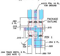
NOTES: 1. TRACE WIDTH IS SHOWN FOR ROGERS RO4350B WITH DIELECTRIC THICKNESS .020" ± .0015"; COPPER: 1/2 OZ. ON EACH SIDE. FOR OTHER MATERIALS TRACE WIDTH MAY NEED TO BE MODIFIED. 2. BOTTOM SIDE OF THE PCB IS CONTINUOUS GROUND PLANE.
