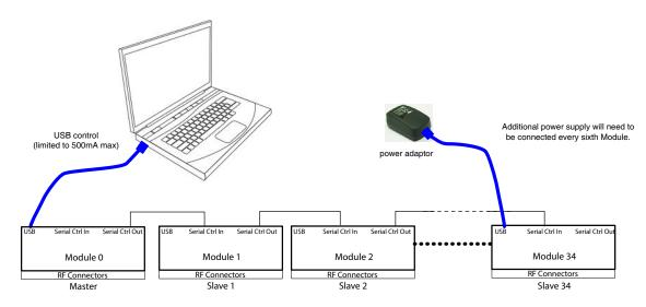
Connections between modules will be made using the serial in/out ports with the module connected to the PC as a master and all others as slave modules. All control will be through the master module (address zero) which is the only one communicating with the PC. Serial control out port of each module should be connected to the serial control in port of the next module. Power will be supplied from the PC via the master module up to a maximum of 500mA.
