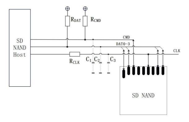
RDAT and RCMD (10K~100 k $\Omega$ ) are pull-up resistors protecting the CMD and the DAT lines against bus floating when SD NAND is in a high-impedance mode.
