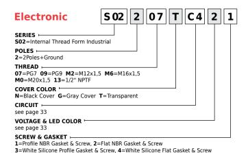
**mPm**® Field Attachable **DIN Valve Connectors**
