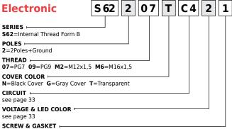
1=Profile NBR Gasket & Screw, 2=Flat NBR Gasket & Screw
