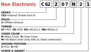
1=Profile NBR Gasket & Screw. 2=Flat NBR Gasket & Screw
