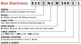
1=Profile NBR Gasket & Screw, 2=Flat NBR Gasket & Screw  ${f 3}=$  White Silicone Profile Gasket & Screw,  ${f 4}=$  White Silicone Flat Gasket & Screw  ${f T}=$  Profile NBR Gasket + IP67 Fixing Screw
