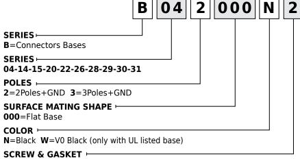
**Note:** UL listed part number identified by adding suffix SA at the end of the nomenclature in conjunction with UL material (W for black and T for transparent) e.g. B142000W2SA
