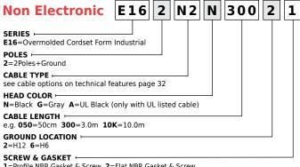
1=Profile NBR Gasket & Screw, 2=Flat NBR Gasket & Screw **3=**White Silicone Profile Gasket & Screw, **4=**White Silicone Flat Gasket & Screw **P=**NBR Integrated Gasket Assembled + IP67 Screw
