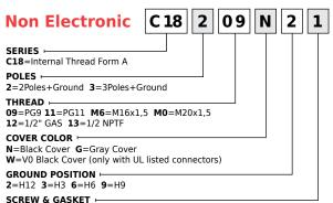
1=Profile NBR Gasket & Screw, 2=Flat NBR Gasket & Screw
