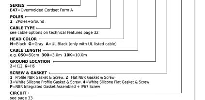
Note: UL listed part number identified by combining UL listed cable with UL overmolding material e.g. E152A3A30011
