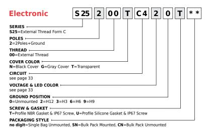
mPm® Field Attachable DIN Valve Connectors
