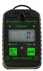
The Inspector features a large LCD readout, positive click buttons, a durable waterproof case, lanyard loop and rugged attachment clip.
