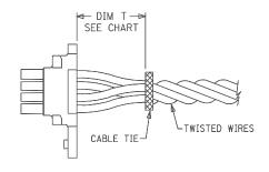
The "T" dimension defines a "free" length of wire, or a length of wire that is not subject to significant bias by external factors such as a wire tie, wire twisting, or other means of bending or deforming of the wires that repositions them from their natural relaxed state or location where they enter the housing. Wires are to be dressed in such a manner to allow the terminals to float freely in the pocket.
